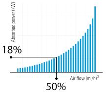
Lambda SKY together with EC fans offer automatic air flow control as standard, either by maintaining a constant flow rate as the site conditions change (progressive fouling) or even better by allowing the flow rate to be modulated according to the required comfort conditions.
