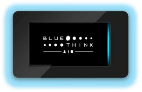
The graphic terminal is a 4.3" touch screen panel. The electronic technology featured and the 65.000 colour display help manage high quality images and advanced functions. The touch screen panel is also designed for easier man-machine interaction as it makes screen browsing much more user-friendly.
