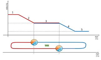
A simplified diagram representing this functionality is shown in the graphs above. RAT represents the return temperature from the environment.ASS instead it is the supply air setpoint. WM is the working mode
