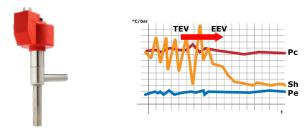
The graph above illustrates the improvement achieved in the controller and in the superheating value (Sh), in parallel with the performance of the evaporation (Pe) and condensing (Pc) pressures, in cases where an electronic valve (E2V) is used.
