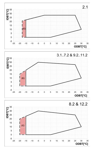
**ODBT:** Temperature of the external air that strikes the condensing coil (dry bulb)
