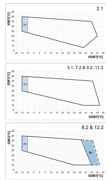
**ODBT:** Temperature of the external air that strikes the condensing coil (dry bulb)
