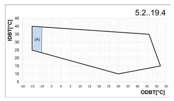
**ODBT:** Temperature of the external air that strikes the condensing coil (dry bulb)
